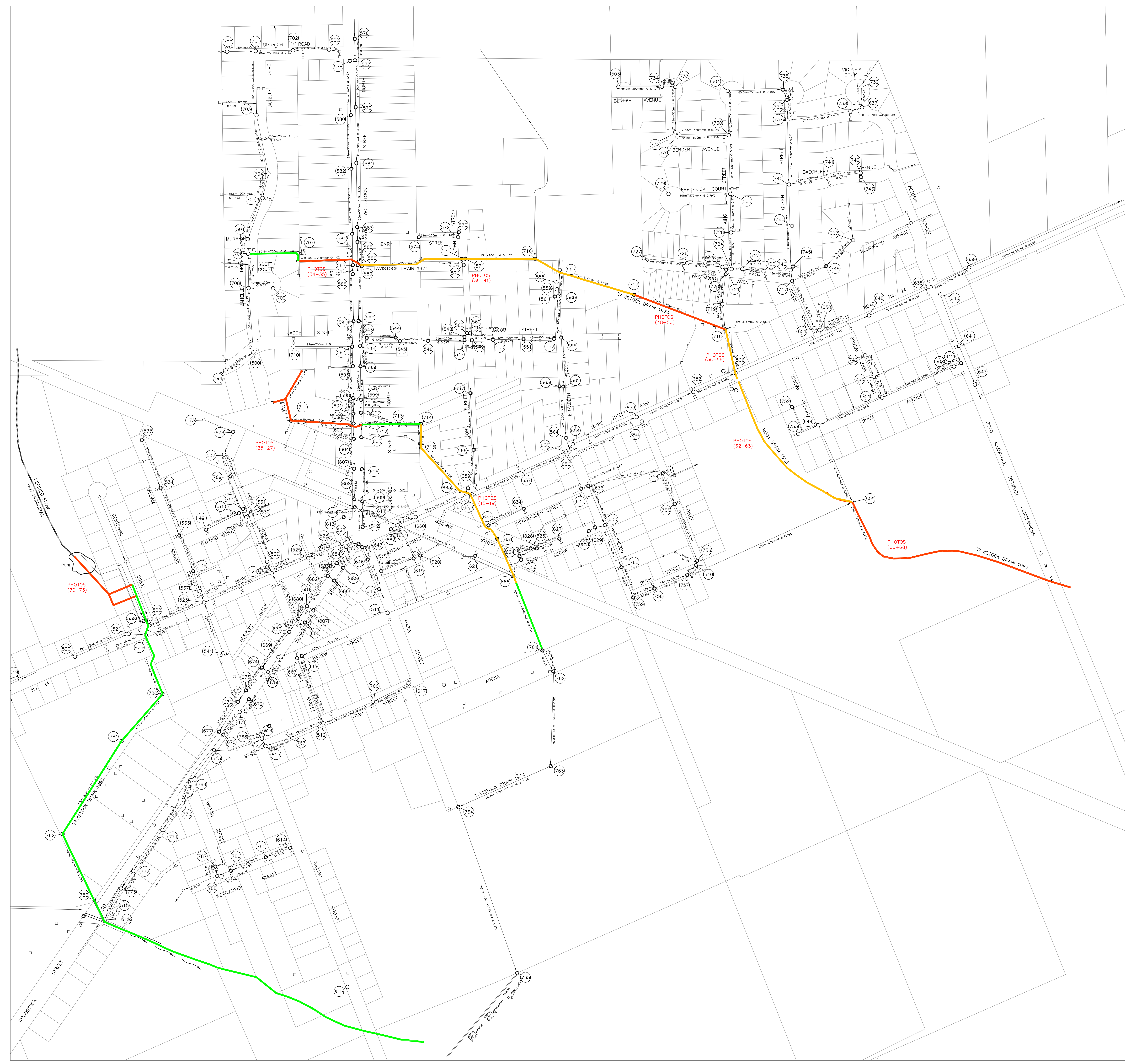
FIGURE 6 TOWNSHIP OF EAST ZORRA-TAVISTOCK TAVISTOCK MASTER STORM SYSTEM DRAINAGE PLAN EXISTING MAJOR OVERLAND FLOW ROUTE
