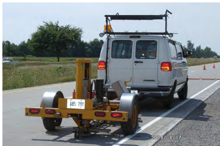
Figure 3-1. Photograph of a Falling Weight Deflectometer.
